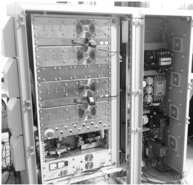
Fig. 19. Experimental power converter. Two three-phase full-bridge CCS050M12CM2 converters are in parallel for the DC/DC stage and two more for the four-wire inverter.
