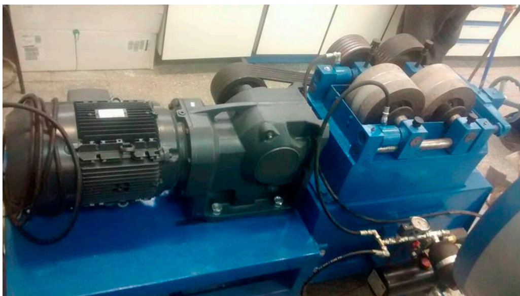
Figure 1. Roll crusher transformed into a high-pressure grinding roller with a 15 kW engine and full hydraulic piston system.
