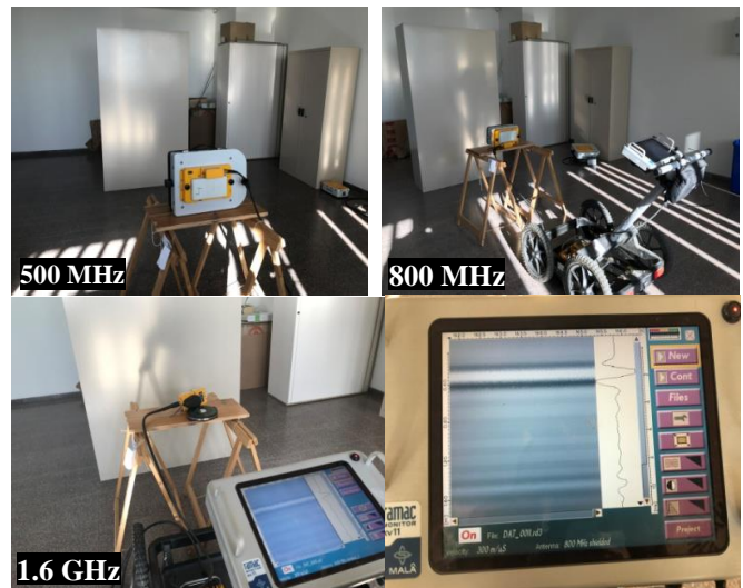
Fig. 2. GPR data acquisition for the zero-time position test using three antennas (500 MHz, 800 MHz and 1.6 GHz).
