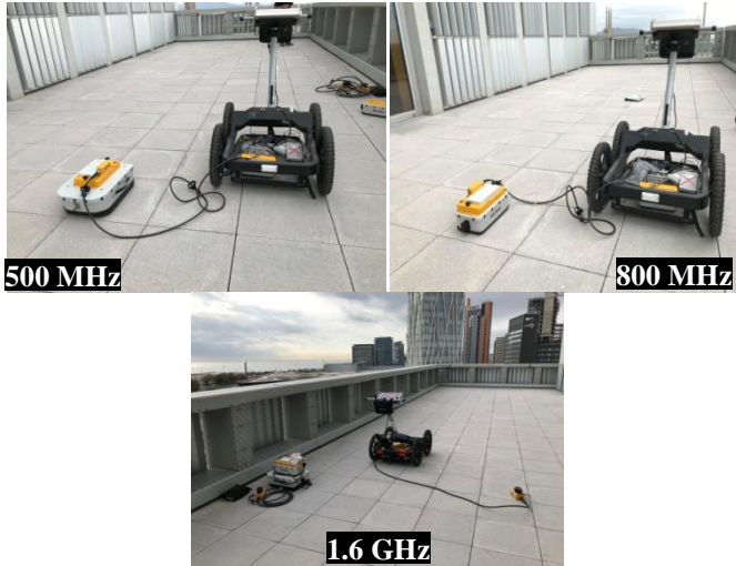
Fig. 1. Radar data acquisition in a concrete floor with 500 MHz, 800 MHz and 1.6 GHz GPR antennas, for the stability tests.
