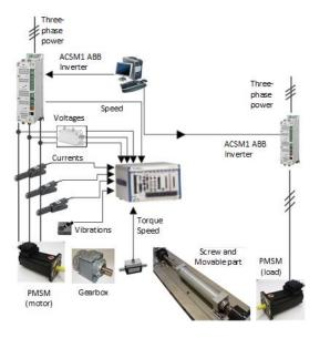
Fig. 2. Experimental test bench used to validate the proposed diagnosis methodology.
