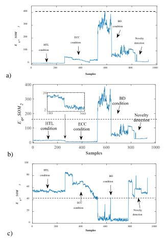
**Fig. 7.** Resulting quantization errors during the assessment of all the considered conditions, that is, HLT, ECC, DB and DEM through: a)  $SOM_1$ , b)  $SOM_2$  and c)  $SOM_3$ .
