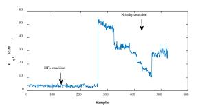
**Fig. 3.** Quantization error performed during the evaluation of the HLT and ECC conditions through the *SOM*<sub>1</sub> model which belong to the initially known condition (healty condition).
