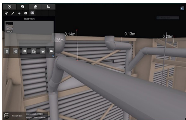
Fig. 7 Measurements placed between model elements in VR. A measurement tool in the software allows users to measure distances in the model and leave dimension marks. A user is seen using the tool and placing dimension by HTC Vive joysticks
