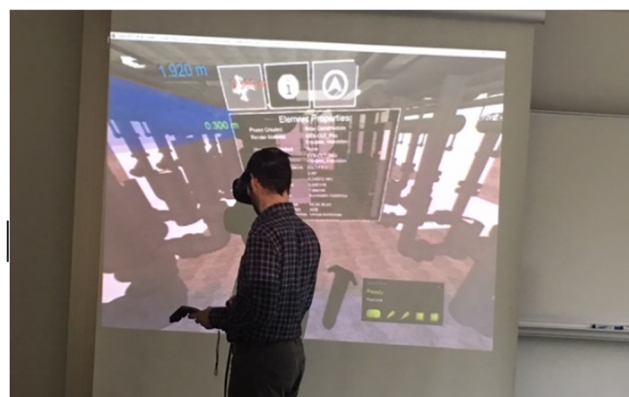
Fig. 7 Measurements placed between model elements in VR. A measurement tool in the software allows users to measure distances in the model and leave dimension marks. A user is seen using the tool and placing dimension by HTC Vive joysticks
