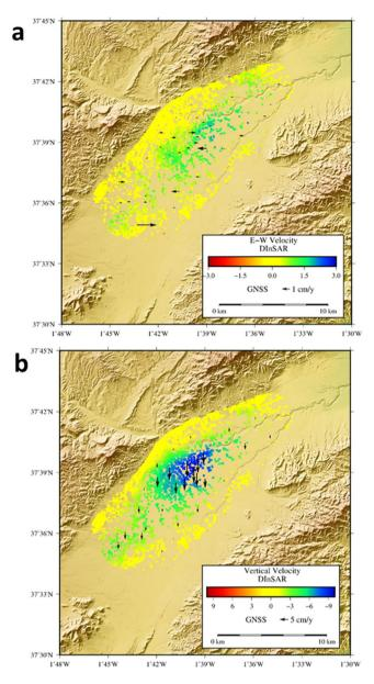
**Figure 5.** East-West and Vertical displacements obtained by A-DInSAR. (a) Horizontal (East-West) and (b) vertical (Up-Down) displacement rates estimations obtained by decomposition of the LOS detected velocity using ascending and descending orbits. GNSS displacements are also plotted with arrows to compare. Results are shown for the period November 2015 - February 2017. GMT software was used to create this figure<sup>75</sup>.
