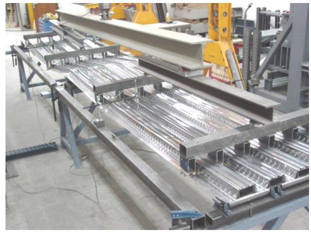
Figure 6. Test set-up for two span bending or continuous deck tests.
