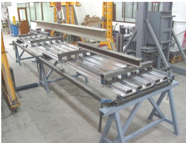
Figure 6. Test set-up for two span bending or continuous deck tests.
