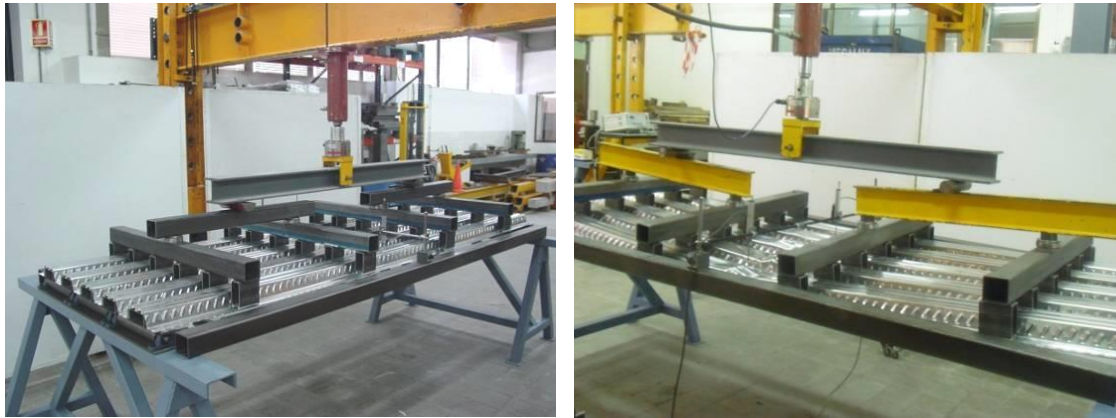
Figure 4b. General views of simply supported deck a) test configuration and b) after collapse.
