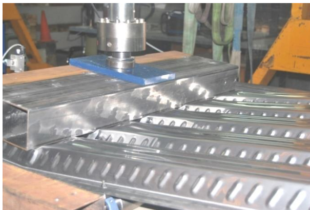
Figure 11. Views of a) end support test configuration for u=40 mm, b) general view of failed deck for u=40 mm, c) detailed view of the collapse of the deck and d) failure of the end support section.
