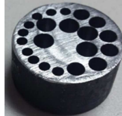
Fig. 1. C45E carbon steel drilled test tube for measuring machinability using different drills.
