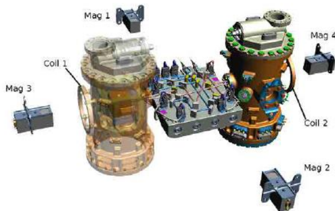
Fig. 8 : The four tri-axial fluxgate magnetometers in the payload of LISA Pathfinder. The TMs (solid gold cube) are located at the centre of each electrode housings (cubic structures) placed inside the vacuum enclosure (cylinders) [3]
