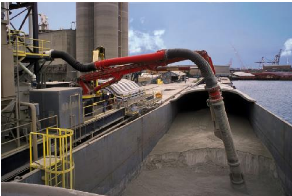
Figure 24. Pneumatic system in an unloading operation suctioning cement from a bulk carrier. Source: https://www.conveyorspneumatic.com
