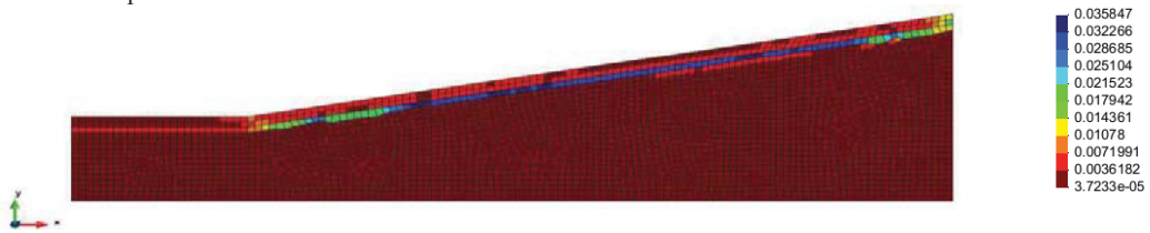
Fig. 6. Calculated plastic deviatoric strains in Ancona slope.
