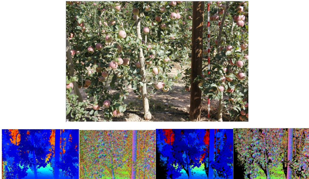
Figure 13. Top picture is the source. Center are depth maps (photometric left – geometric right). Bottom, normal maps (photometric left - geometric right)
