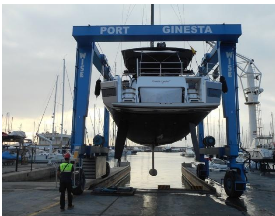
Figura 82. Travelift 75 tn Port Ginesta. – Font: Port Ginesta
