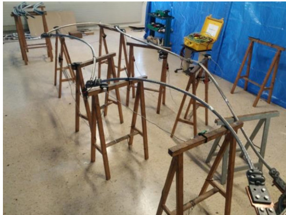
Figure 2.12: Temperature rise tests. Test loop composed of HTLS conductors and S285ZTLS T-type mechanical substation connectors.
