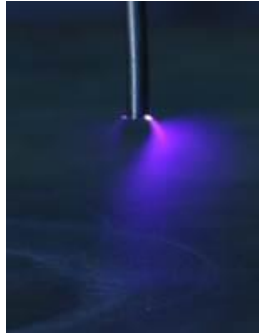
Figure 3.1: Inception of positive corona and streamer.
