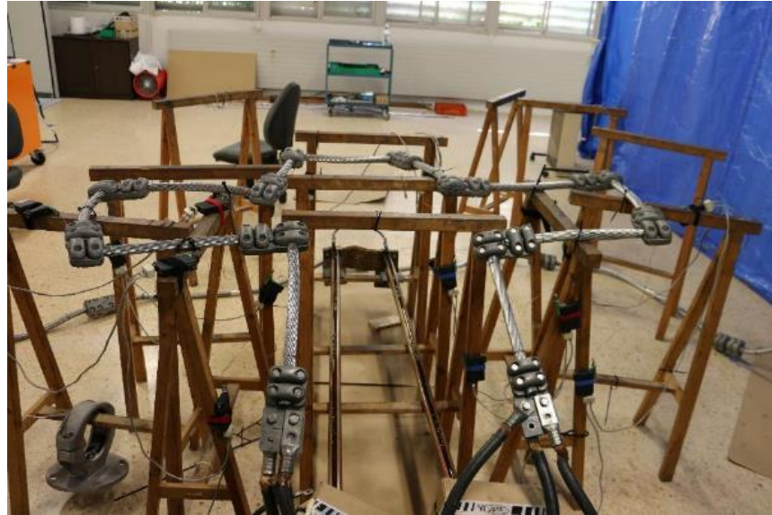
Figure 4.5: Experimental loop tested in AMBER facilities of the UPC to conduct the SSADT test.
