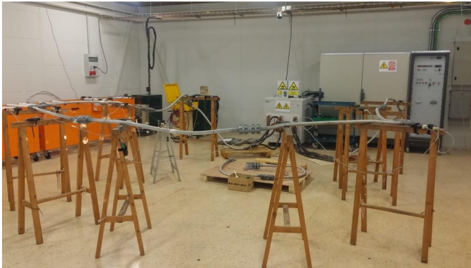
Figure 2.3: Temperature rise test assembly for substation connectors
