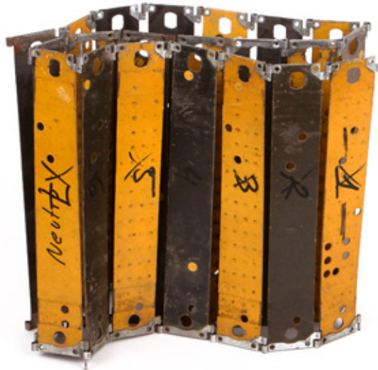
IV-2-4 / For Jacquard looms, punchcard based weaving program
