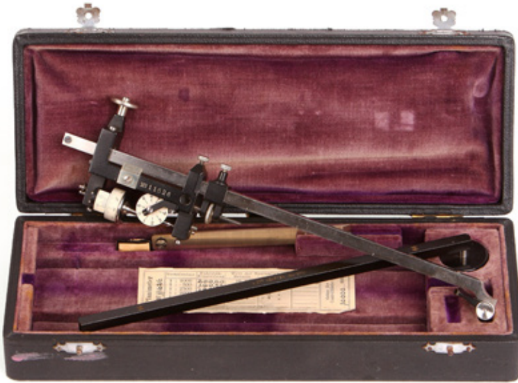
V-4-1 / Planimeter, for the automatic computation of areas
