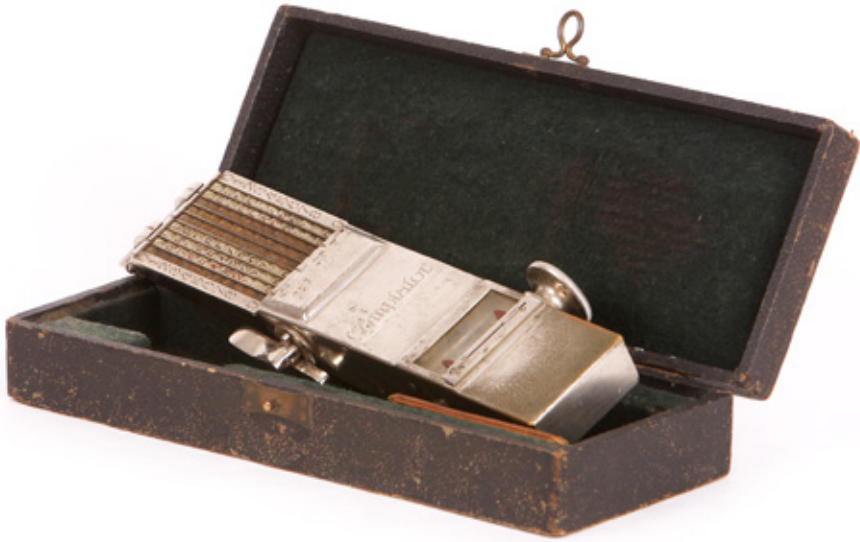
I-4-1 / Comptator... the portable manual accumulator
