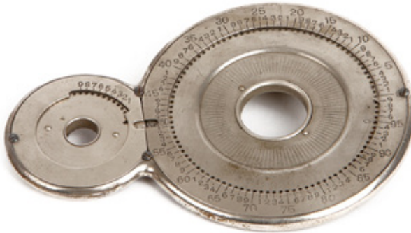
III-4-1 / Figure-8-Adder, the eight fitted for the hand
