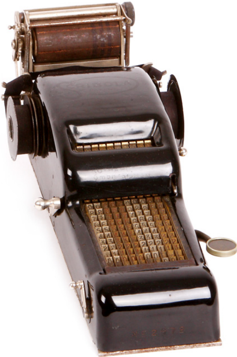
III-4-3 / Scribola adder-lister, the adder than prints
