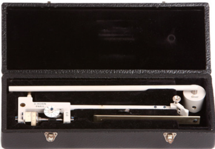
V-4-2 / Morin planimeter, mechanizing mathematical integration
