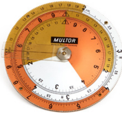
III-3-3 / Multor, pocked multiplying wheel
