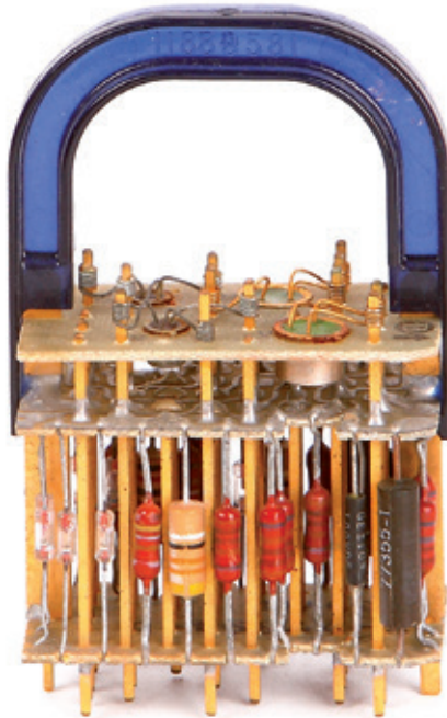
VI-4-2 / Burroughs functional pluggable board by hardware
