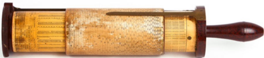
V-3-1 / Fuller desktop spiral rule, for logarithmic supercomputing
