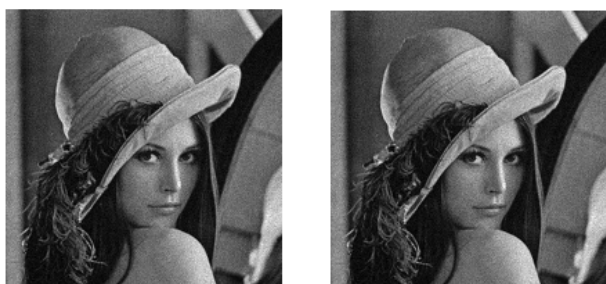
Figure 8. The corresponding processed images. Left: by using the average filtering ( SSIM=0.6834 ). Right: by invoking our first approach ( SSIM=0.6720 ).
