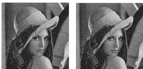
Figure 5. The corresponding processed images. Left: by using the average filtering ( SSIM=0.4174 ). Right: by invoking our first approach ( SSIM=0.4091 )
