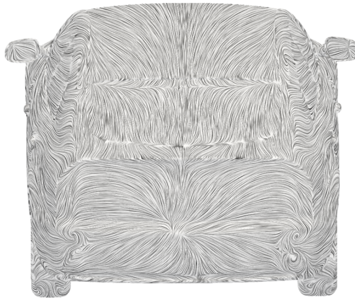
Figure 7: Streamlines for the average flow
