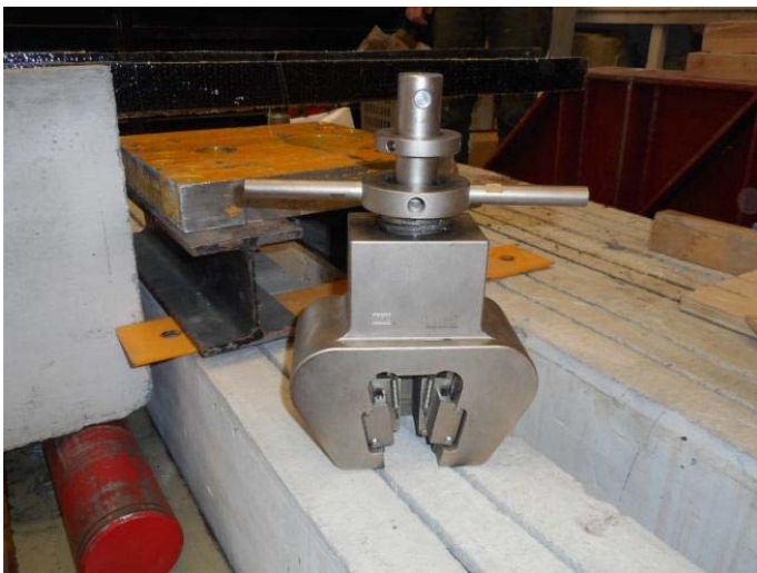
Figure 7. Grips for clamping and pulling of the laminates
