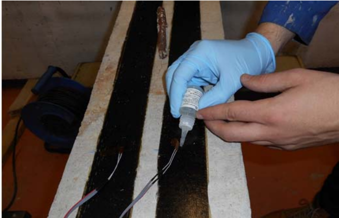
Figure 5. Strain gage installation on the BFRP laminate
