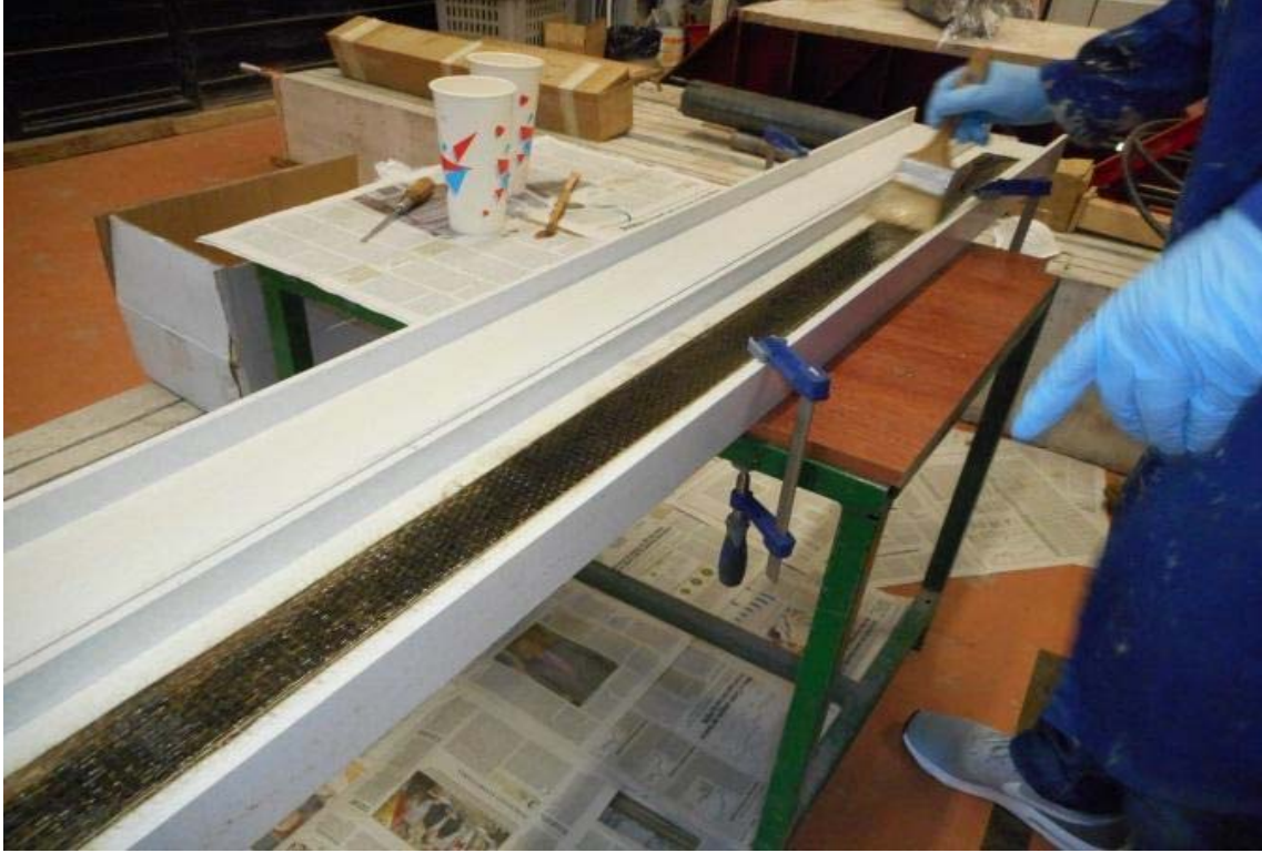
Figure 4. Hand lay-up manufacturing of basalt composite FRP
