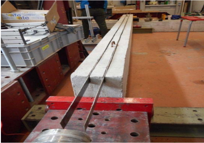
Figure 6. Positioning of laminates inside slits
