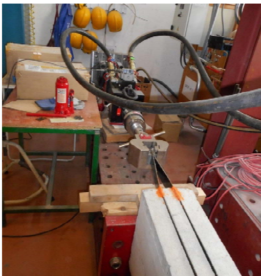
Figure 8. Pulling system with actuator
