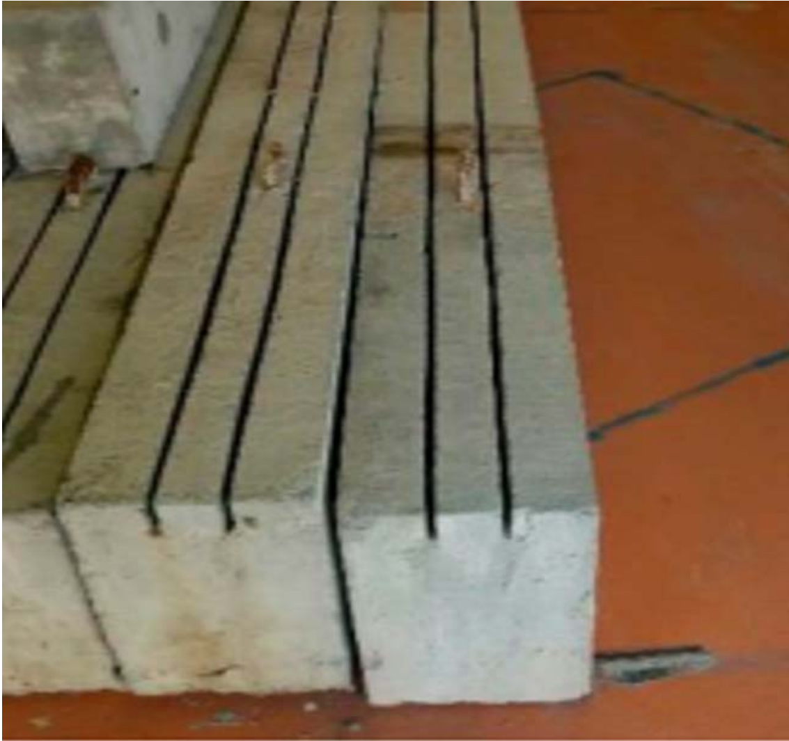
Figure 2. Detail of slits for embedding FRP laminate
