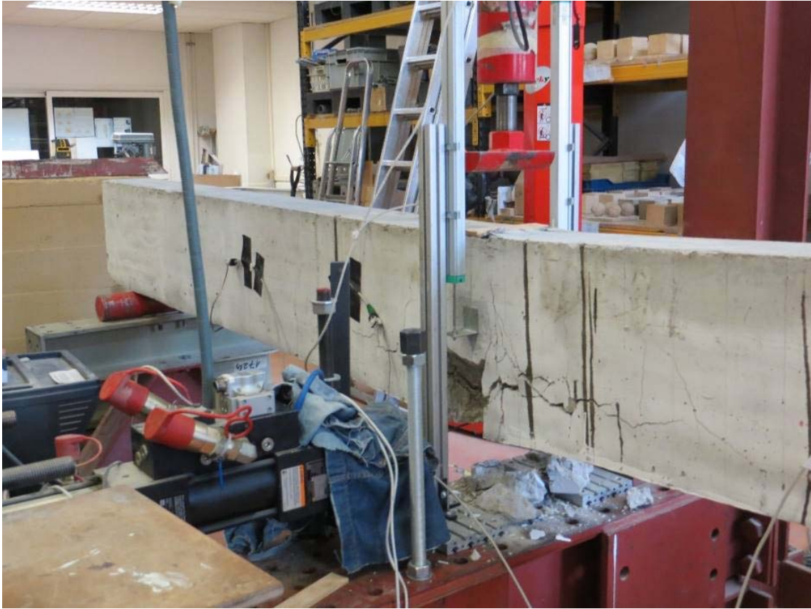
Figure 17. Failure of the FRP-control beam
