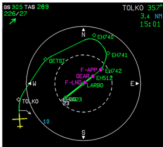
Fig. 7: Optimised trajectory by DYNAMO as seen in the Navigation Display
