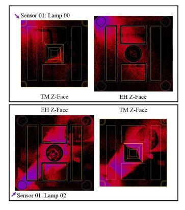
FIG. 5: The distribution of absorbed UV light on the lower z-faces of the flight sensor. Top: Illumination provided by lamp 00 which is aimed at the test mass. The primary test mass surfaces are shown on the left while light reflected onto the housing surfaces can be seen on the right. Note that the primary light falls directly on the test mass corner with little reflected
