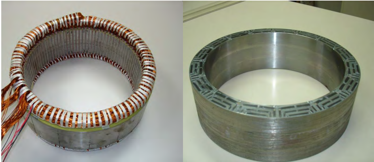
Figure 116. The stator and rotor obtained with the proposed methodology
