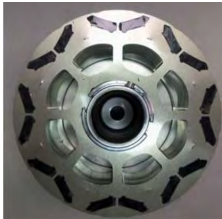
Figure 1. Rotor of Prius (2010) [12]
