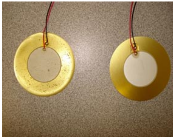
Fig. 3.1 Surface bounded PZT
