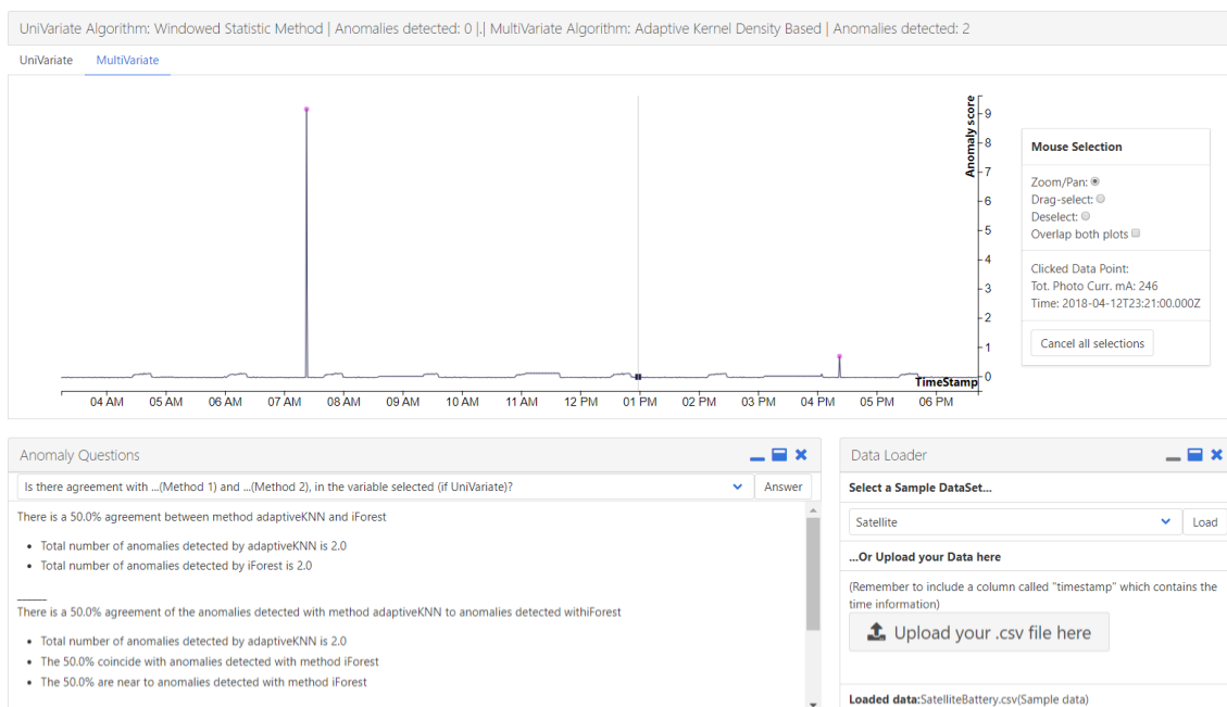
Figure 17: Adaptive Kernel Density Based Algorithm Anomaly scores and Agreement with iForest. Two spikes appear on the anomaly score, corresponding to the anomalies introduced.
