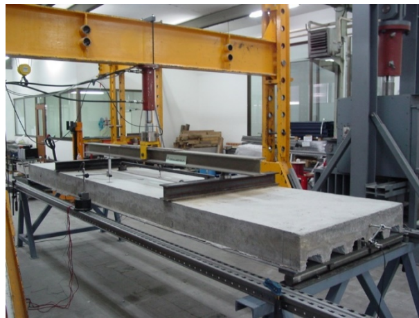
Figure 7 General view of the experimental setup for composite slabs
