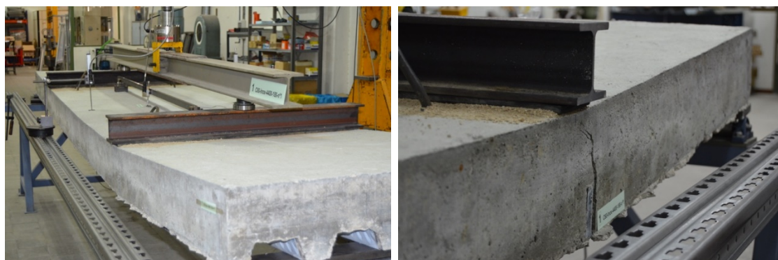
Figure 9 Long slabs after slip failure
