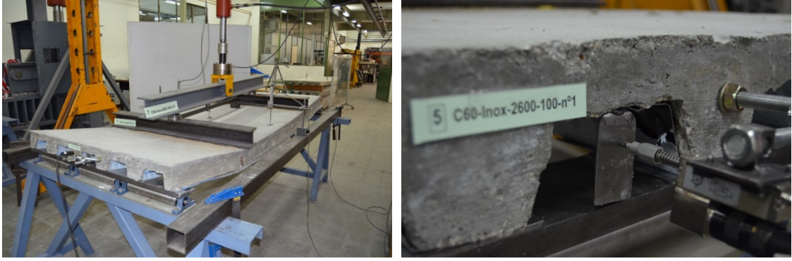
Figure 12 Short slab after longitudinal shear failure
