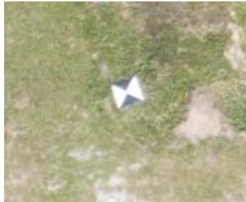
Figure 1 50x50 cm GCP as seen in an aerial picture taken at 120m AGL
