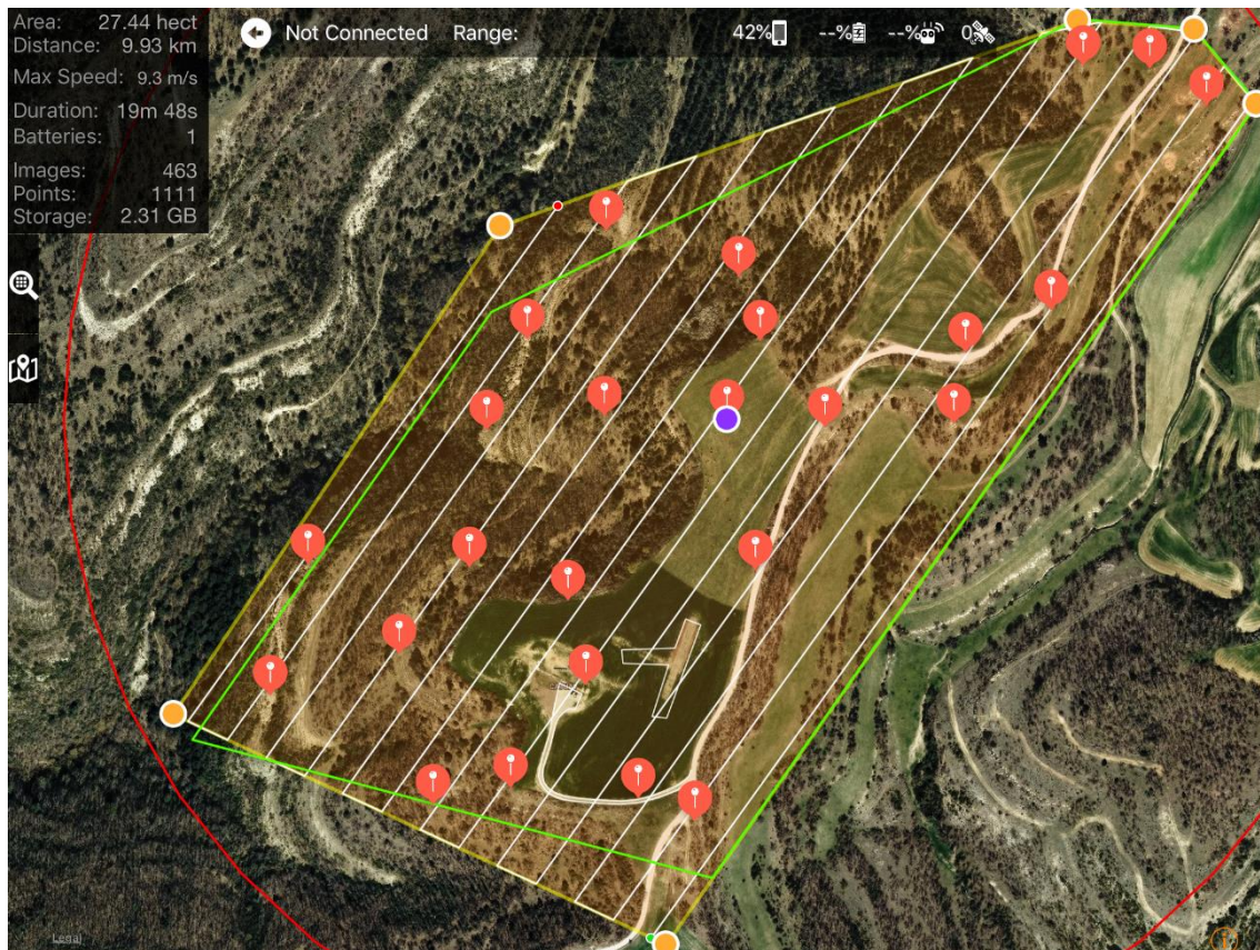
Figure 10 DMP flight path in white colour. Note that not all GCPs are visible in the image.
