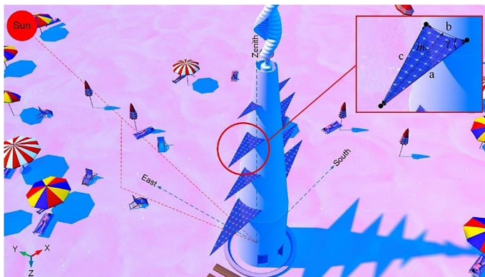
Fig. 5 The three-dimensional model environment for shading analysis
