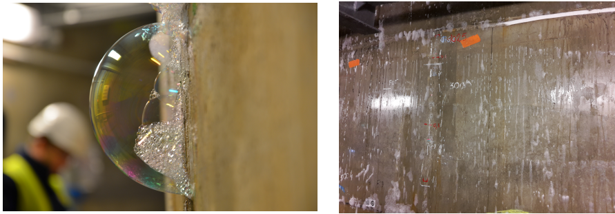
Figure 5.16: Images taken during the leakage tests [24]
