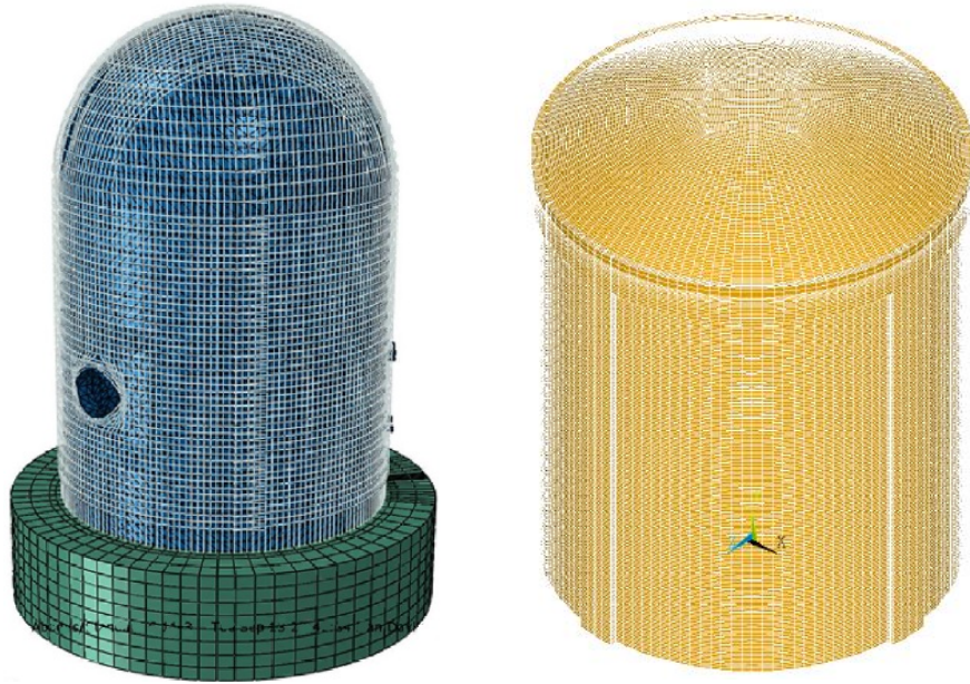
(a) FE mesh of a containment building analysed using Abaqus [40] (b) Containment building model where truss smeared elements are used for rebars [43]
