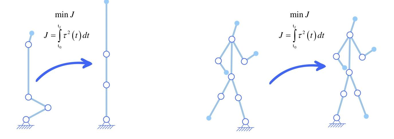
Differences in optimization performance were observed comparing different dynamic formulations and type of coordinates. The fact that we obtained a lower number of iterations when using natural coordinates and explicit formulations in more complex models could be explained by the constant mass matrix [3].
