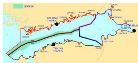
Figure 30: Area of GOFREP, the mandatory Ship reporting System of the Gulf of Finland. -Font: Development Process of the Gulf of Finland Mandatory Ship Reporting System. [104]
