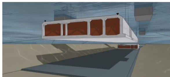
Figure 6: Fehrmanbelt, Immersion of the modules with pontoons.- Font: https://femern.com/en [37]
