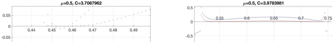
Figure 4.12: Zoom for the first intersection of W_-^u with \Sigma_{r_2} for \mu = 0.5 . We overlap r_1 (red) with the cross product \mathbf{r} \times \dot{\mathbf{r}} (blue) for different values of \mu . We appreciate two collisions for C = C_2 at normalized time \theta_1 \approx 0.451 and \theta_2 \approx 0.458 . The case C = (C_1 + C_2)/2 does not show collisions.
