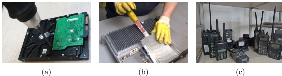
Figure 1.1: (a) Bottom view of a hard drive being disassembled. (b) GSM amplifier being disassembled. (c) Several handie-talkie models being displayed.
