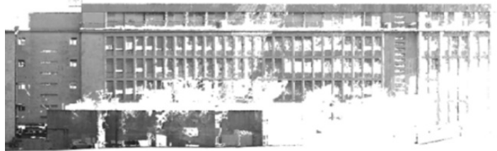
Figure 3. Taking and managing a point cloud generated from laser scanners for the construction of buildings (RA). Author: E. Redondo
