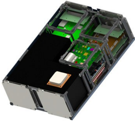
Fig. 1. 3 CAT-2 interior 3-D model. The white patch is the L1/L2 dual-polarization antenna to receive the direct signal.
