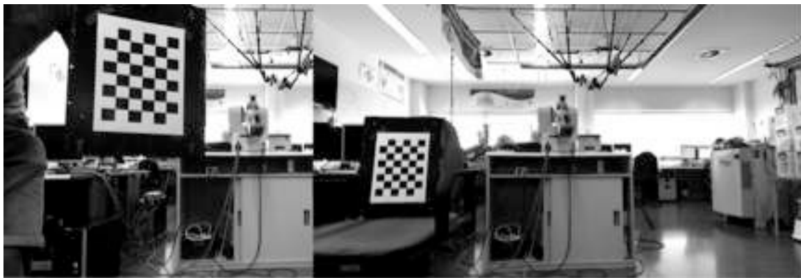
Fig.15: Calibration images for Kinect v2
