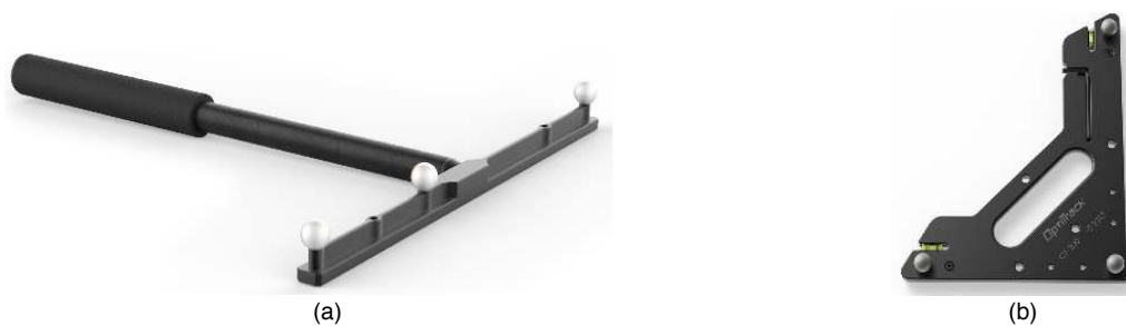
Fig.19: Instruments for the Optitrack Calibration and reference system setup
