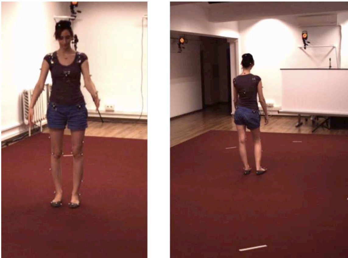
Fig.25: Placement of the reflectors over the human body.
