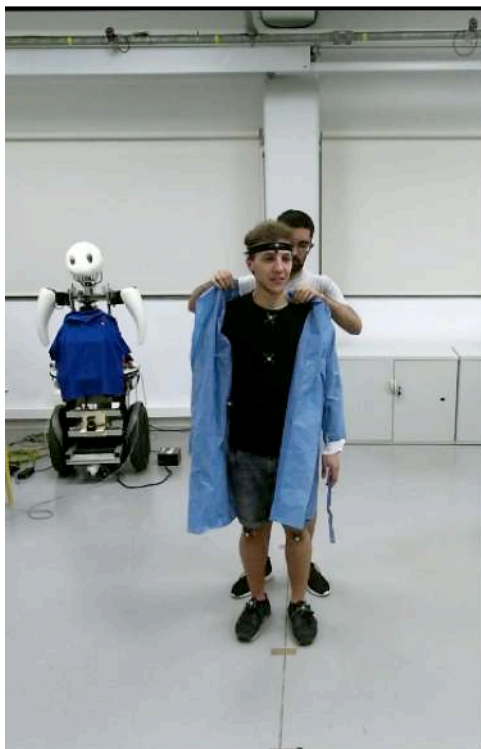
Fig 30: Example where we can see the occlusions in the OptiTrack when the jacket covers the arms
