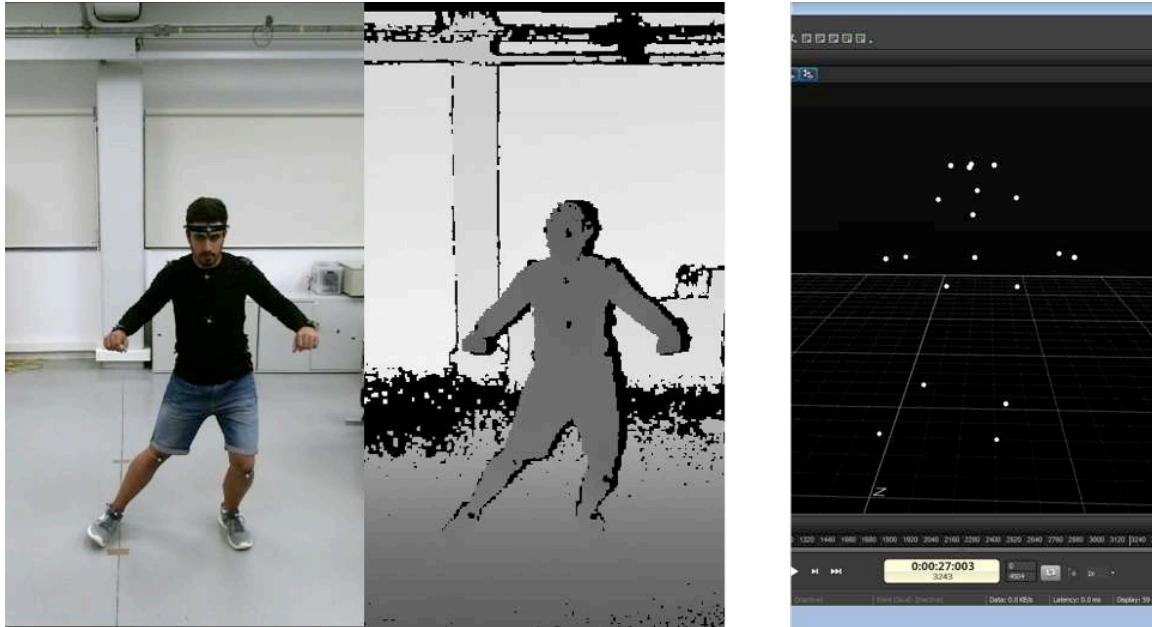
Fig.34: Associate images (RGB and Depth images of the Kinect and the “map” of OptiTrack)
