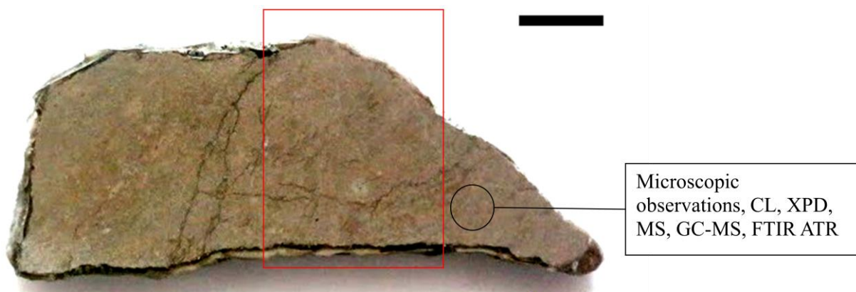
Applied methods on sample 2/4/A , scale: 1 cm ( sample 2/4 ; polished surface). Abbreviations: CL – Cathode luminescence microscope, XPD – X-ray powder diffractometry, CL – Cathode luminescence microscope, MS – mass spectroscopy, GC-MS – Gas chromatography mass spectroscopy, FTIR ATR – Attenuated total reflectance Fourier transform infrared spectroscopy
