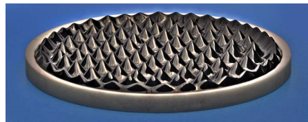
FIG. 1. (Color online) Rosensweig peaks of the magnetic fluid type EMG 909, Ferrotec Co., at a supercritical induction B > B_c in a vessel with diameter of 120 mm. A movie showing the formation of Rosensweig patterns can be accessed at Ref [9].
