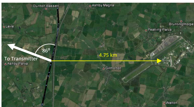
Fig. 5 Satellite image of the Bruntingthorpe target area with the flight path of the aircraft shown (black line), and the distance and direction to the transmitter (white line), and the distance to the air field (yellow line)
