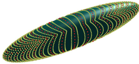
FIG. 5. Sketch of the nearest-neighbor discretization of a prolate spheroid. Here, the red dots show the force discretization, with a disjoint quadrature set shown in light green. (Figure in color online.)
