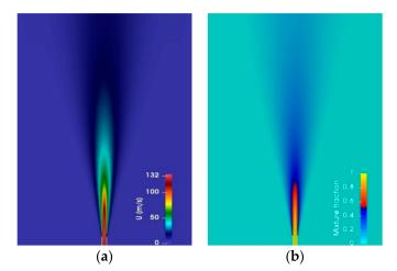
**Figure 6.** Contour plots from ESF/FPV simulation for Oxyfuel flame B3: (a) mean velocity, (b) mixture fraction.
