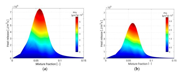
**Figure 1.** Production rate of heat release in the mixture fraction space coloured with source term of the PV. (a) distribution of heat release in Flames A1, B3 tables, (b) distribution of heat release in Flame A3 table.
