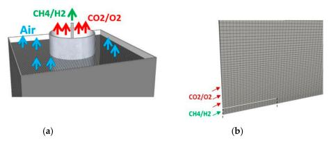
**Figure 3.** Oxyfuel configuration (**a**) Description of the Oxyfuel configuration according to the experimental set up in reference [28]. (**b**) Inlets part from the 2D numerical block structured grid.
