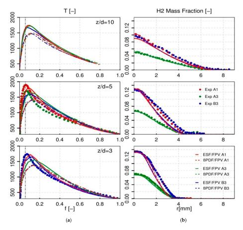
Figure 10. Mean temperature profile in mixture fraction space (a) and  $H_2$  mass fraction (b) results from ESF/FPV simulation with 48 SFi at different axial positions for flame cases A1, A3 and B3 in comparison with β-PDF results and Raman/Rayleigh data from [28].
