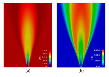
**Figure 5.** Contour plots from ESF/FPV simulation for Oxyfuelflame B3: (a)Temperature distribution, (b) meanCO<sub>2</sub> mass fraction.
