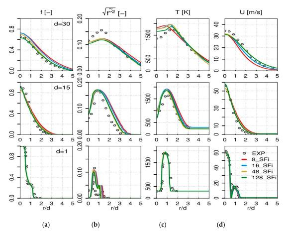
**Figure 4.** Comparison between experimental data for Flame-D [16] and RANS numerical results for different numbers of SFi at different axial positions; d = 1, d = 15 and d = 30, (a) mean mixture fraction, (b) rms of mixture fraction, (c) mean temperature and (d) mean velocity.
