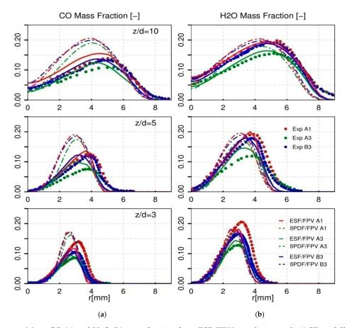
Figure 11. Mean CO (a) and  $H_2O$  (b) mass fraction from ESF/FPV simulation with 48 SFi at different axial positions for flame cases A1, A3 and B3 in comparison with β-PDF results and Raman/Rayleigh data from [28].
