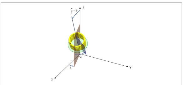
**Figure 3.** Spool geometry used to calculate the phase-corrections due to the rotation of the Earth. The x-axis is always pointing South, the z-axis is normal to the surface of the Earth and the y-axis is pointing to the East. The photons enter the spool in a plane defined by the angle  $\alpha_i$ , where i is indexing the corresponding fiber spool.
