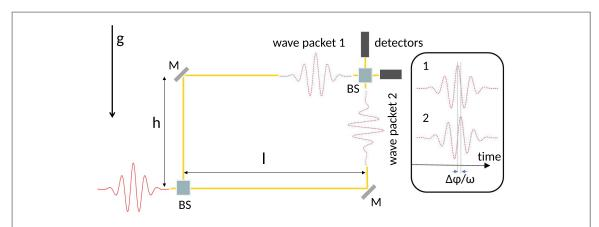
**Figure 1.** Schematic of a conventional Mach–Zehnder interferometer of area A = lh placed vertically inside Earth's gravitational field. A beam splitter (BS) transforms a single photon into a coherent superposition between the two possible arms. The wave function evolves along two different paths and arrives at the merging beam splitter at the same time but slightly shifted in phase due to the presence of a gravitational potential.
