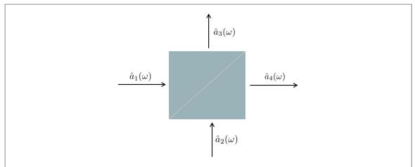
**Figure B1.** Representation of a symmetric lossless beam splitter showing the annihilation operators associated with the input and output fields.
