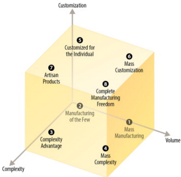
Figure 3 The three-axis model of product manufacturability shows that product design must address complexity, required iterative customizability and required volume to be readily manufacturable.
