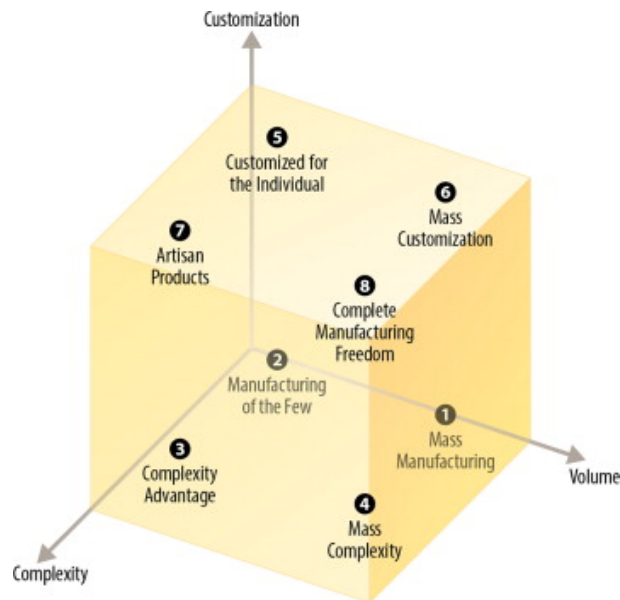
Figure 3 The three-axis model of product manufacturability shows that product design must consider complexity, required iterative customizability and required volume to be readily manufacturable.
