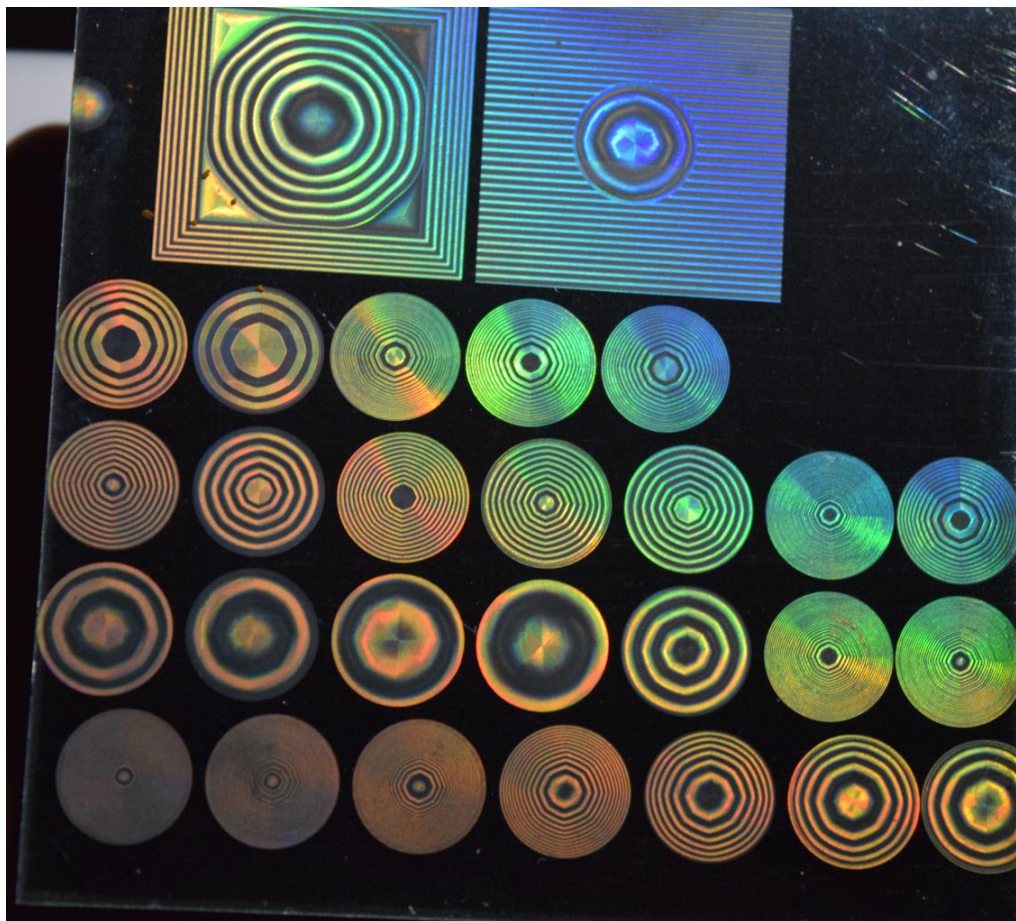
Figure S2. Fields of radial periodic pattern of ripples orientations processed with different stepper motor rotation to beam scanning speed ratios.
