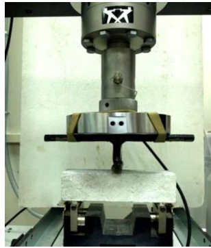
211 212 Figure 5: Failure deformation test setup using INSTRON machine
