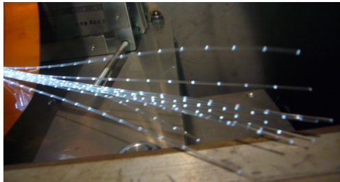
Figure 6: A bundle of clear fibres. Each fibre has 18 notches to supply the LED light to the 18 strips in a row of scintillators.
