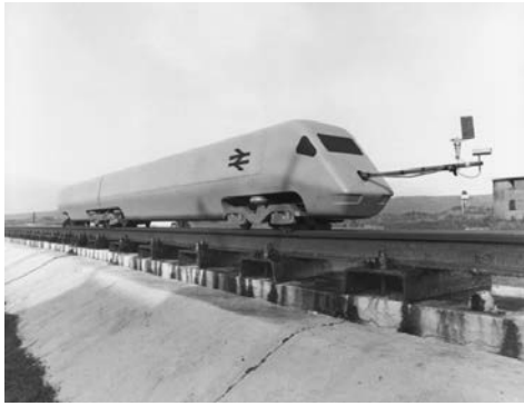
(a) The Pendine experiments using 1/5 th scale APT (photograph from National Railway Museum)
