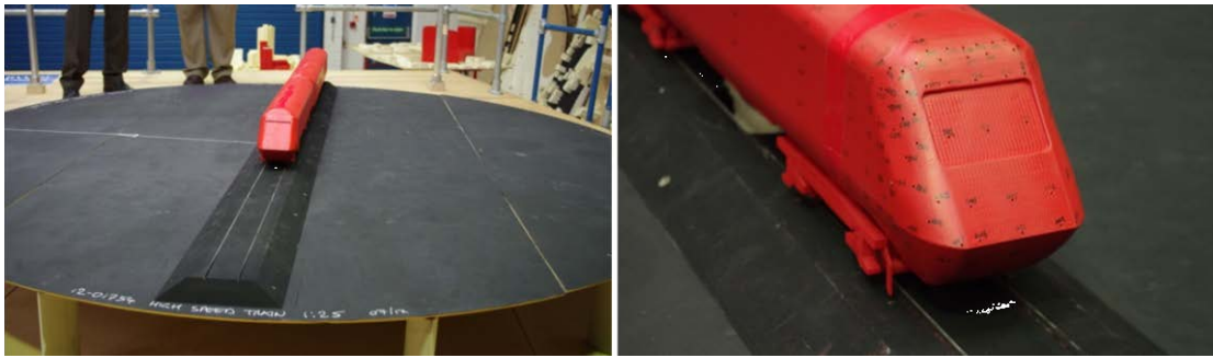
(a) The wind tunnel model and setup
