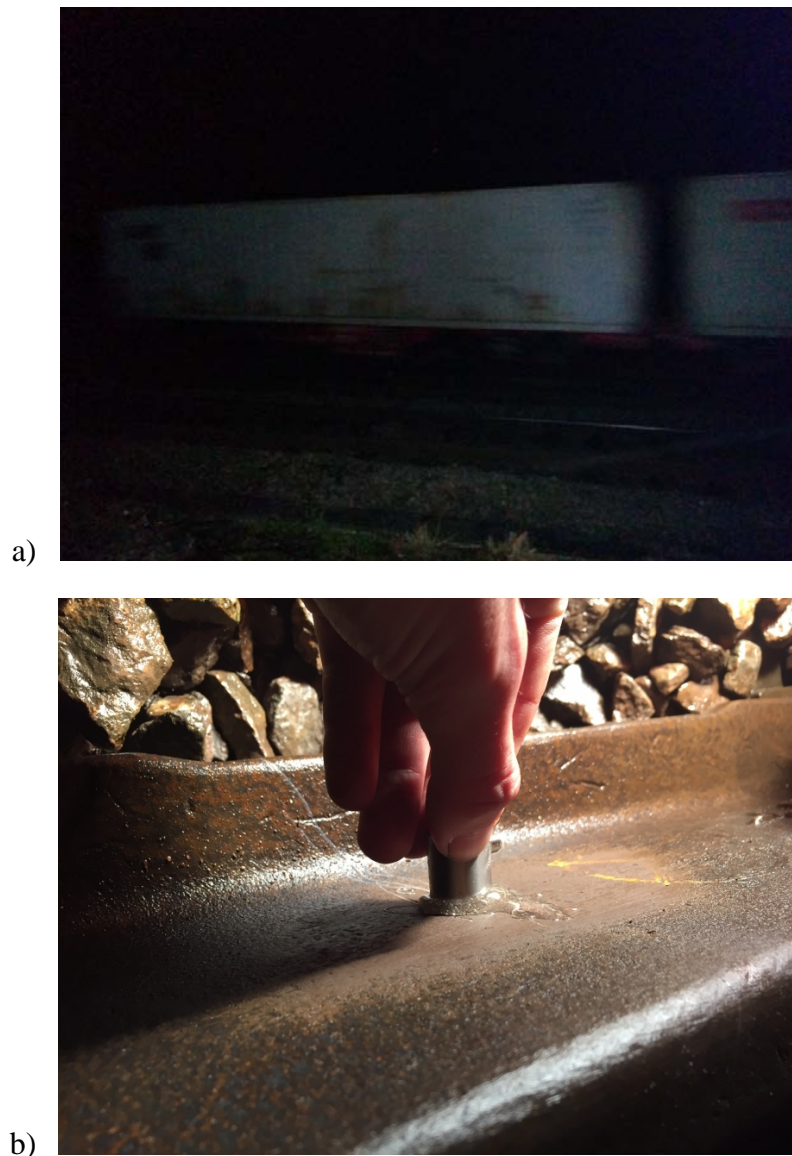
Figure 3: Photographs showing: a) the indicative traffic at the instrumented Hatton crossing and b) AE sensor installation with Araldite.
