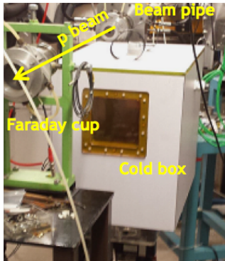
Figure 4. The temperature controlled chamber, the beam line with beam direction indicated, and the Faraday cup at the setup.
