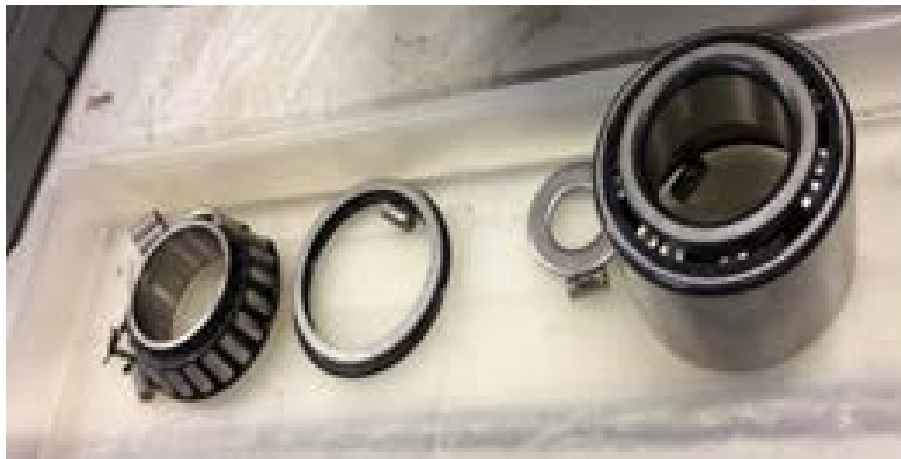
Figure 2: Example of a double-row tapered roller bearing used in the test rig laboratory experiments.
