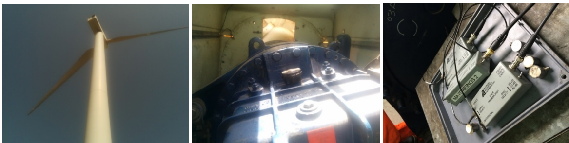
Figure 10: The 850 kW TERN Energy wind turbine gearbox instrumented in Crete together with the AE sensors and pre-amplifiers employed for its instrumentation.
