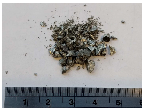
Figure 8 Hydrogen treated Alloy 1 material after 20 tonne compression. (a) Front, (b) side.
